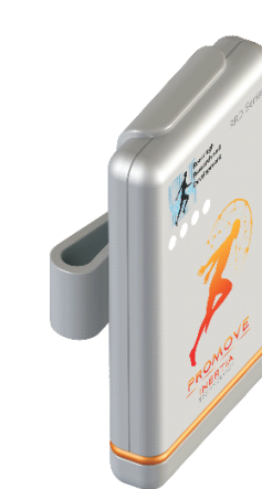
Figure 1: The Promove3D contains a 3D accelerometer with output in counts per minute, according to Bouten et al. (1997). To be worn at the hip.
