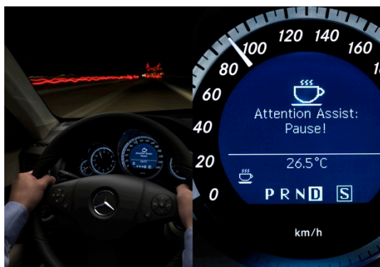
Figure 5 – Drowsy driver alert system
