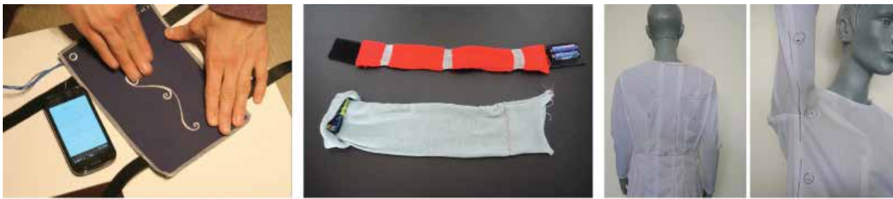
a) Measuring pressure, feedback with audio b) Measuring stretch & touch, different yarns c) Canvas to determine sensor locations
