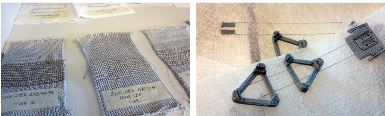
Figure 1: Examples of conductive yarns and 3D printed structures.
